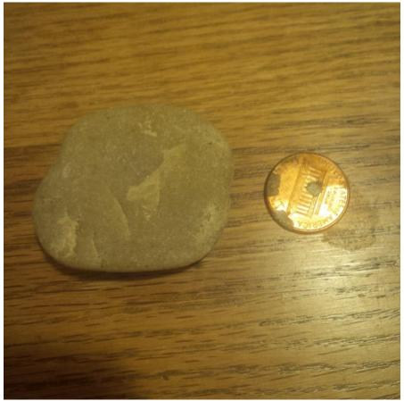
Photo 1- Sample of rounded rock taken from pile at base of crack in the west sidewall of the East Culvert. This is presumed to be original backfill material.
