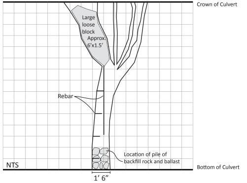
JACOBS ASSOCIATES Cracks in East Culvert 10/11/2013
